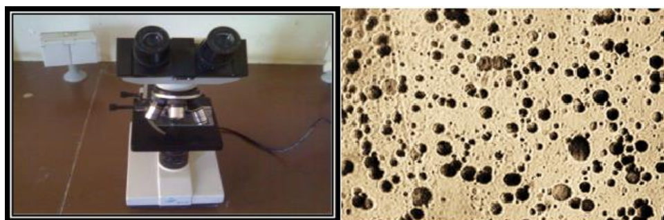
Fig. 2. Optical microscope and etched tracks in RL- 115 in Cihan tea.
