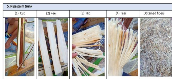
Fig. 6. How to separate the fibers from Nipa palm trunks.
