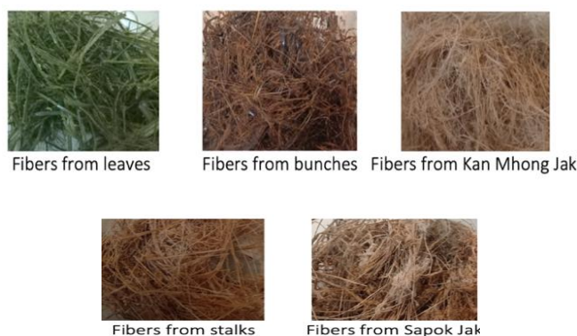
Fig. 9. The fibers obtained from all five parts of Nipa palm after soaking in Softener HSB and then soaking in Texamina.
