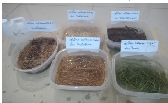
Fig. 7. The sample image of the fibers when soaking in the Softener HSB.
