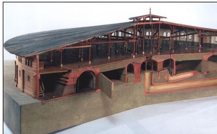
Fig. 12. Cross-section of the Friedrich Hoffmann's "Ring Kiln".
