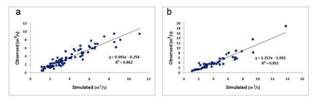
**Fig. 5.** Scatter plot of river streamflow for (a) calibration period (2001-2007) and (b) validation period (2008-2011).
