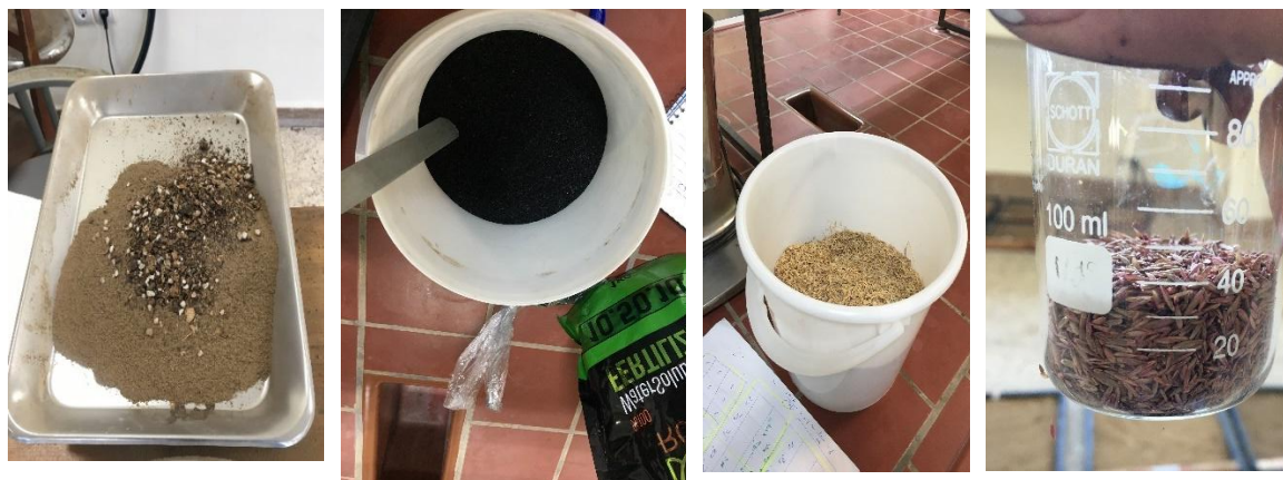
Fig. 3. Preparation of NBH treatment (from left to right: rice husk, biochar, sawdust, and grass seed, respectively).
