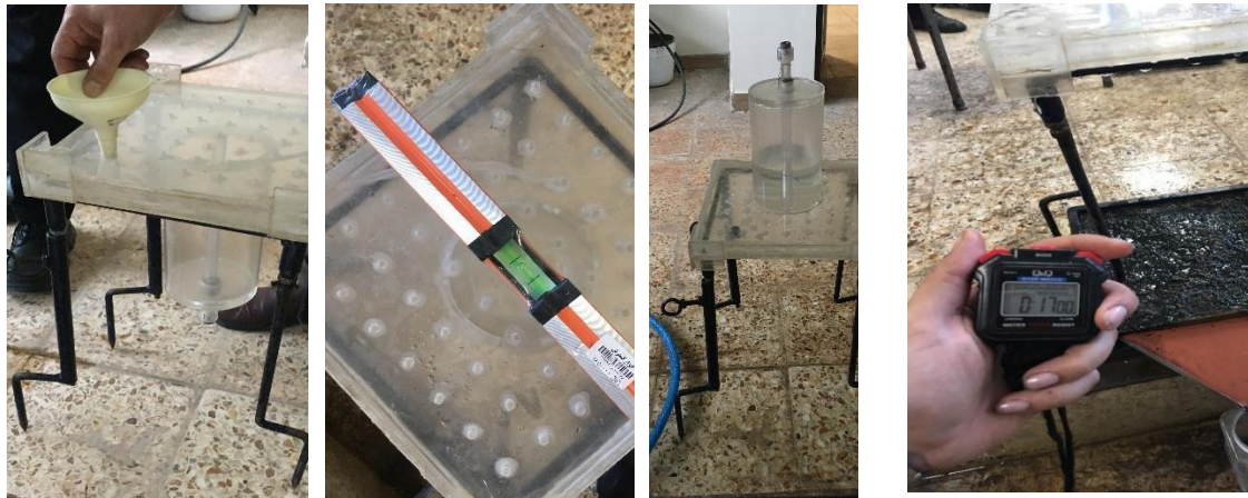
Fig. 5. Preparing the rain simulator and recording the necessary data for each sample.
