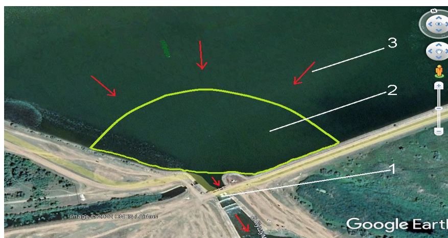
Fig. 2. Section of the water area in front of the spillway, at a distance of 150 m from the gate valve, dangerous for fish and juveniles (1 - dam spillway; 2 - section of the water area dangerous for fish and juveniles; 3 - direction of flow).
