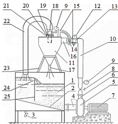
**Fig. 3:** Schematic diagram of an experimental hydrocyclone pumping unit; 1: tank; 2: guide rail; 3: drainage; 4: pump suction pipe; 5: pump; 6: pump discharge pipe; 7: electric motor; 8: valve; 9: pressure gauge; 10: discharge hose; 11: hydrocyclone; 12: goniometer; 13: nozzle; 14: mounting bolt; 15: bracket; 16: inlet pipe; 17: sand pipe; 18: drain pipe; 19: lock nut; 20: sealing gasket; 21: nut; 22: drain pipe hose; 23: racks; 24: spillway; 25: partition.
