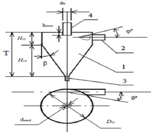
**Fig. 4:** Low-pressure hydrocyclone; T is the height of the cyclone; H<sub>cy</sub> is the height of the cylinder; H<sub>co</sub> is the height of the cone; h<sub>dr</sub> is the depth of immersion of the drain pipe;  $\varphi^\circ$  is the angle of inclination of the inlet pipe along the vertical plane;  $\theta^\circ$  is the angle of inclination of the inlet pipe along the horizontal plane.
