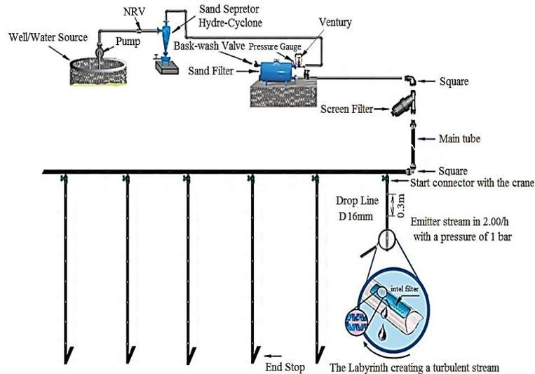
**Fig. 1.** Schematic diagram of the drip irrigation system
