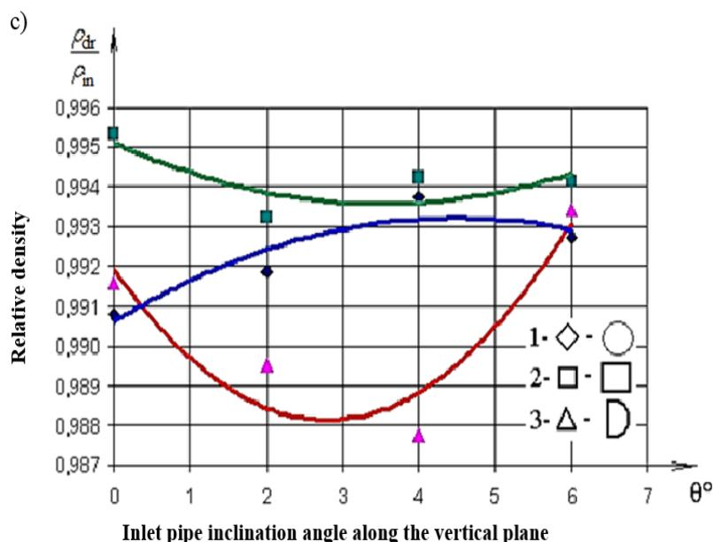
Fig. 9. Dependency graphs for various forms of the inlet hole; a) not immersed drain pipe; b) the drain pipe is immersed to the lower edge of the inlet pipe; c) the drain pipe is immersed up to the interface plane of the cylindrical and conical parts
