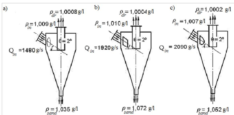
**Fig. 6.** A diagram of the clarification of the treated pulp in a hydrocyclone with various shapes of the inlet section, at  $a_c = 1$ ;  $\theta = 2^\circ$ ;  $\varphi = 0^\circ$ ;  $P = 0.5 \text{ kgf/cm}^2$ ; a) by a circular section of the inlet pipe; b) by a square section of the inlet pipe; c) by a semicircular section of the inlet pipe.
