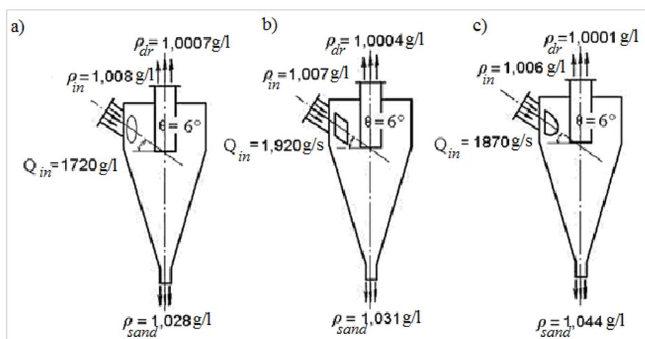
**Fig. 8:** A distribution diagram of pulp consistency in a hydrocyclone with various shapes of the inlet section, at  $a_c = 1$ ;  $\theta = 6^\circ$ ;  $\varphi = 0^\circ$ ;  $P = 0.5 \text{ kgf/cm}^2$ ; a) with a circular section of the inlet pipe; b) with a square section of the inlet pipe; c) with a semicircular section of the inlet pipe.
