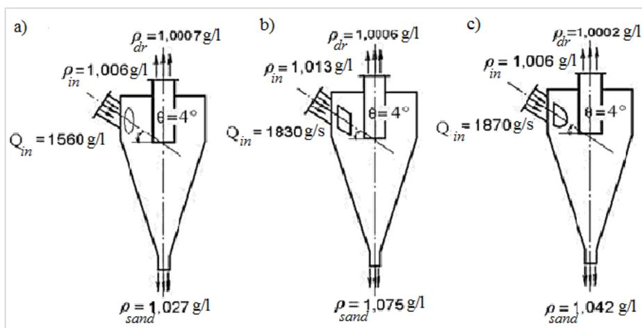
**Fig. 7:** A distribution diagram of pulp consistency in a hydrocyclone with various shapes of the inlet section, at  $a_c = 1$ ;  $\theta = 4^\circ$ ;  $\varphi = 0^\circ$ ;  $P = 0.5 \text{ kgf/cm}^2$ ; a) by a circular section of the inlet pipe; b) by a square section of the inlet pipe; c) by a semicircular section of the inlet pipe.
