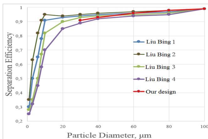
Fig. 10. Comparison of the separation efficiency of four Liu Bing hydrocyclones with that designed in this study at different particle sizes.
