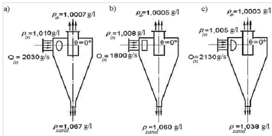
**Fig. 5.** A diagram of the clarification of the treated pulp in a hydrocyclone with various shapes of the inlet section, at  $a_c = 1$ ;  $\theta = 0^\circ$ ;  $\varphi = 0^\circ$ ;  $P = 0.5 \text{ kgf/cm}^2$ ; a) by a circular section of the inlet pipe; b) by a square section of the inlet pipe; c) by a semicircular section of the inlet pipe.
