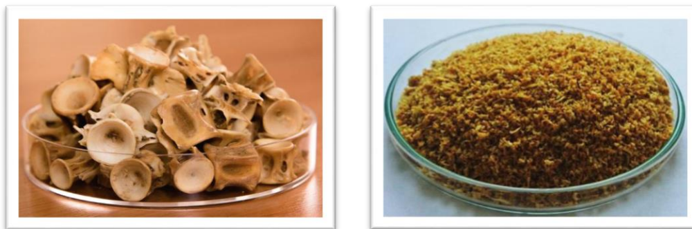
Fig. 1. Bone waste of yellowfin tuna and bone powder prepared therefrom (Photos taken by the authors).
