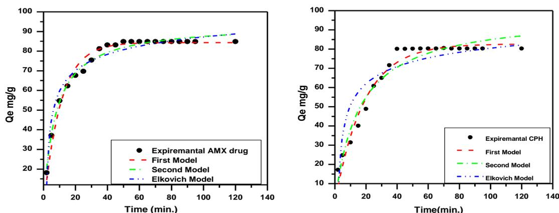
**Fig. 5.** Adsorption rate curve models fitted to experimental AMX and CPH onto SA-Bn-TiO<sub>2</sub> NPs; a) kinetic first order; b) second order; and c) Elovich.
