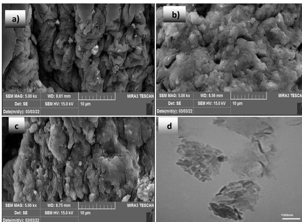
**Fig. 2.** FE-SEM images of (a) SA-Bn-TiO<sub>2</sub> NPs; (d) AMX loaded SA-Bn-TiO<sub>2</sub> NPs; (e) CPH loaded SA-Bn-TiO<sub>2</sub> NPs; and TEM images of (a) SA-Bn-TiO<sub>2</sub> NPs.
