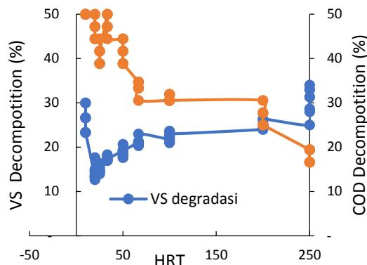
**Fig. 3.** Degradation of organic materials during loading.
