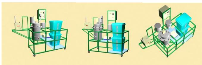
**Fig. 1.** Combination model of biogas and composting in converting organic waste into biogas and compost.
