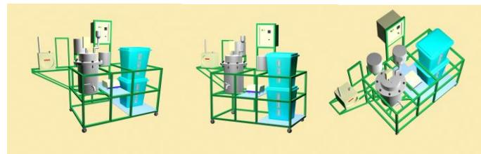
**Fig. 1.** Combination model of biodigester and composter in converting organic waste into biogas and compost.
