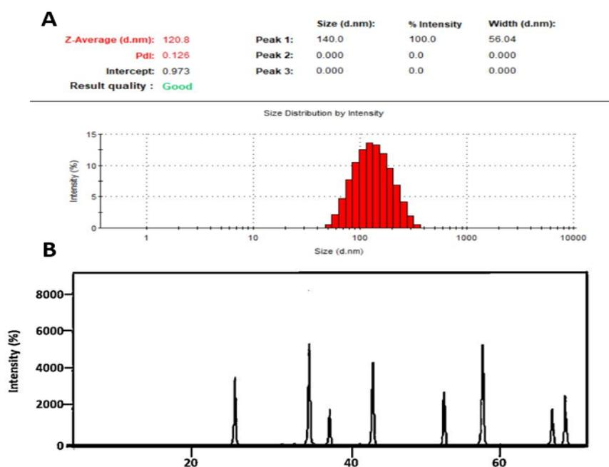
**Fig. 1.** Size measurement images. The  $\text{Al}_2\text{O}_3$ -NPs size using dynamic light scattering (DLS) (A) and crystal structure of the  $\text{Al}_2\text{O}_3$ -NPs with XRD (B).
