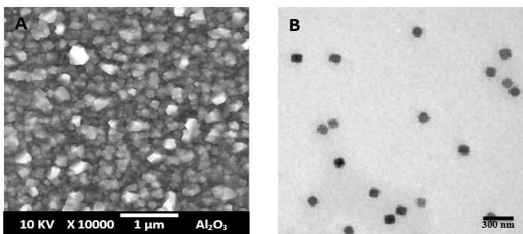
**Fig. 2.** FESEM image of  $\text{Al}_2\text{O}_3$ -NPs (magnification 10 kX) (C); TEM image of  $\text{Al}_2\text{O}_3$ -NPs (D).
