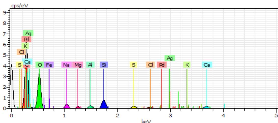
Fig. 6. EDS spectra of *S. portulacastrum* leaf represented interaction between Ag and Pb (100 mg L<sup>-1</sup>).
