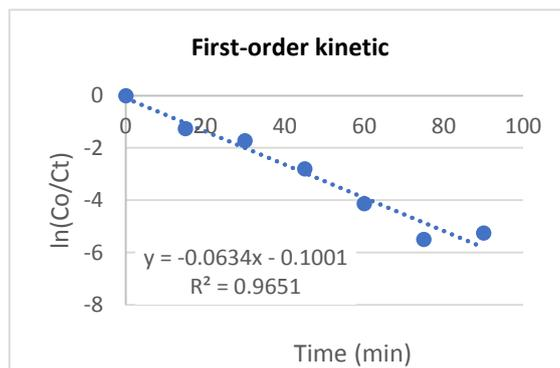
Fig. 9c. Experimental data and the fitted linear equations of 1<sup>st</sup> order kinetic for Cu<sup>+2</sup> adsorption on OPAC.
