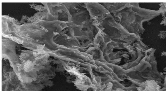
Fig. 1. SEM of orange peel before activation.
