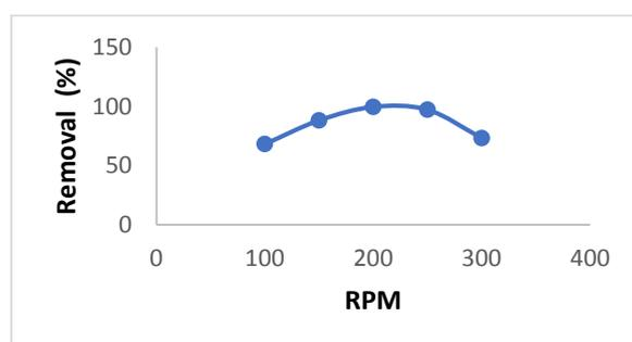
Fig. 5. Effect of RPM on copper (II) removal, pH = 6.5, dose = 0.5 g L<sup>-1</sup>, time = 180min, Cu = 1 mg L<sup>-1</sup>.
