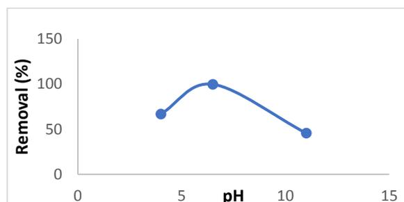
Fig. 3. Effect of pH on copper (II) removal, dose = 0.5 g L<sup>-1</sup>, time = 180 min, Cu = 1 mg L<sup>-1</sup>.
