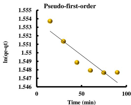
**Fig. 9a.** Experimental data and the fitted linear equations of pseudo 1<sup>st</sup> order for  $\text{Cu}^{+2}$  adsorption on OPAC.
