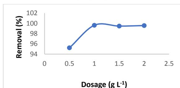
Fig. 4. Effects of doses on copper (II) removal, pH = 6.5, time = 180 min, Cu = 1 mg L<sup>-1</sup>.
