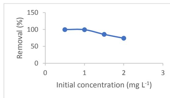
Fig. 7. Effects of initial concentration on removal of copper (II), dose = 0.5 g L<sup>-1</sup>, time = 180 min, pH = 6.5.
