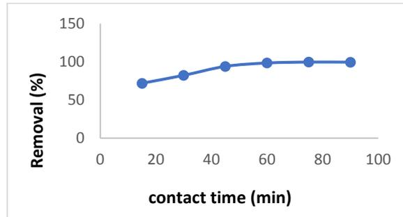
Fig. 6. Effects of contact time on copper (II) removal, pH = 6.5, dose = 0.5 g L<sup>-1</sup>, Cu = 1 mg L<sup>-1</sup>.
