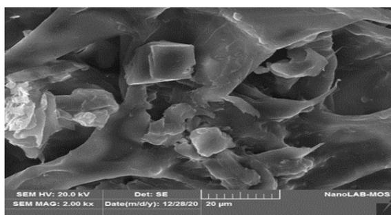
Fig. 2. SEM of orange peel after activation.
