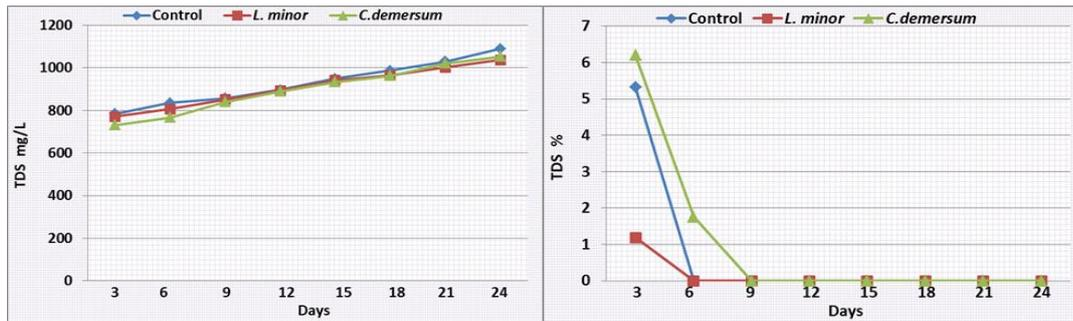
Figs. 4 A-B. Concentrations and rate (%) of bio-removal of TDS ( $\text{mg L}^{-1}$ ) during remediation.
