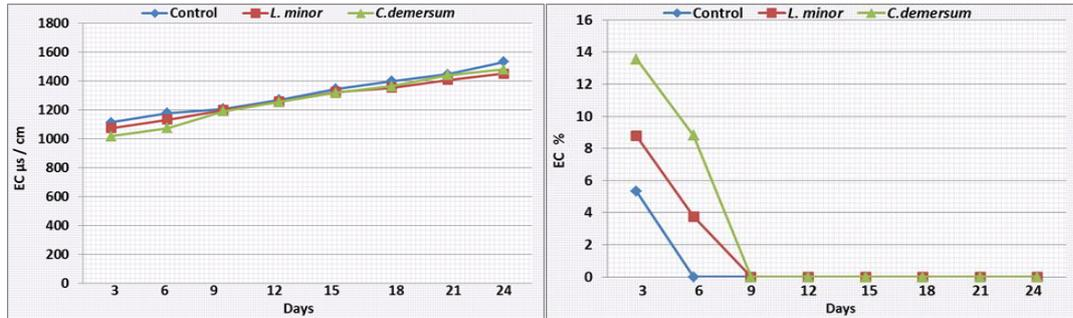
Figs. 3. A-B. Concentrations and rate (%) of bio-removal of EC ( $\mu\text{s cm}^{-1}$ ) during remediation.
