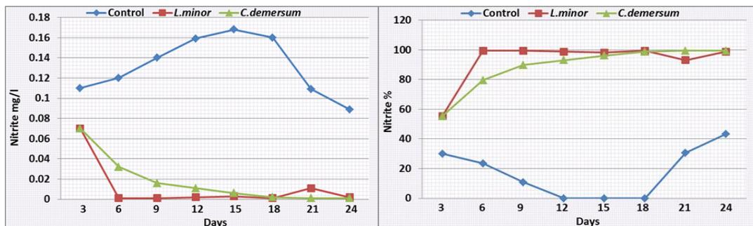
Figs. 6 A-B. Concentrations and rate (%) of bio-removal of nitrite ( $\text{mg L}^{-1}$ ) during remediation.
