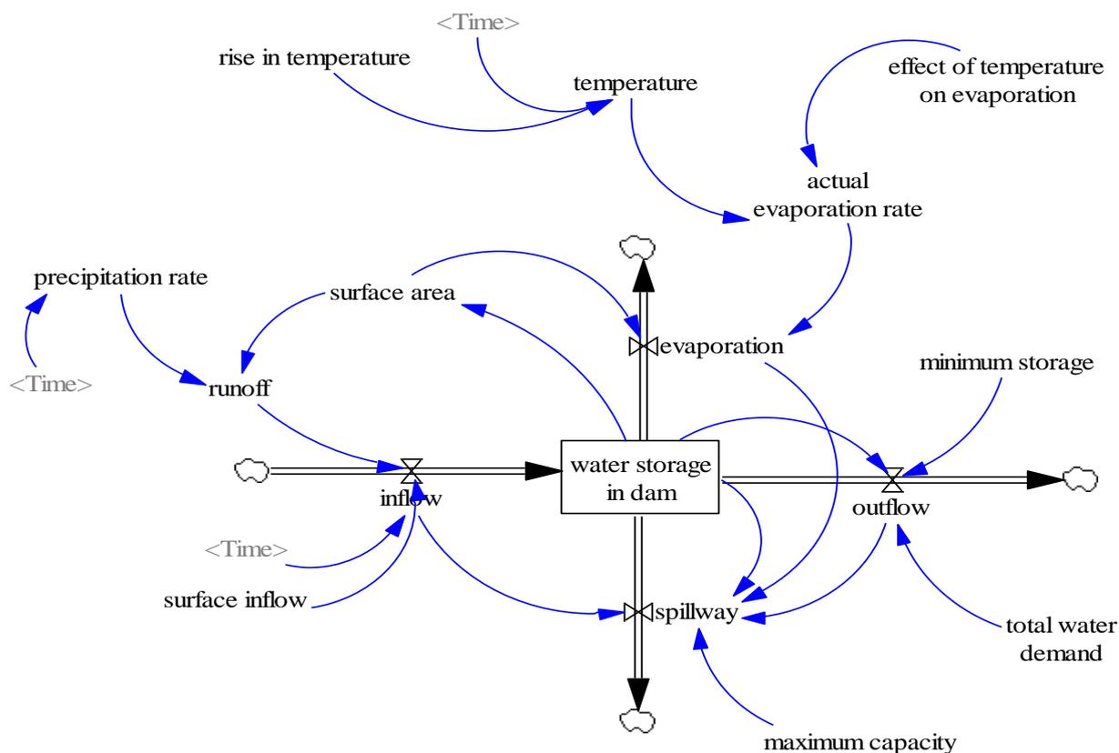
Fig. 3. Water supply stock and flow diagram.
