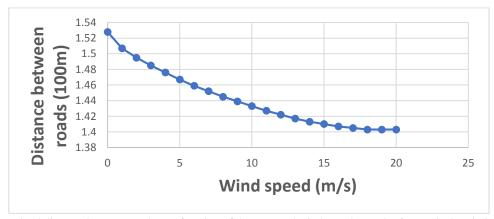
Fig. 5. The optimal distance between roads as a function of the expected wind speed. Result of numerical optimization.
