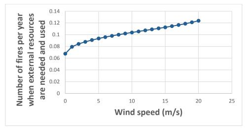
Fig. 6. The expected number of fires per year when external fire fighting resources are needed and used as a function of the expected wind speed. Result of numerical optimization.
