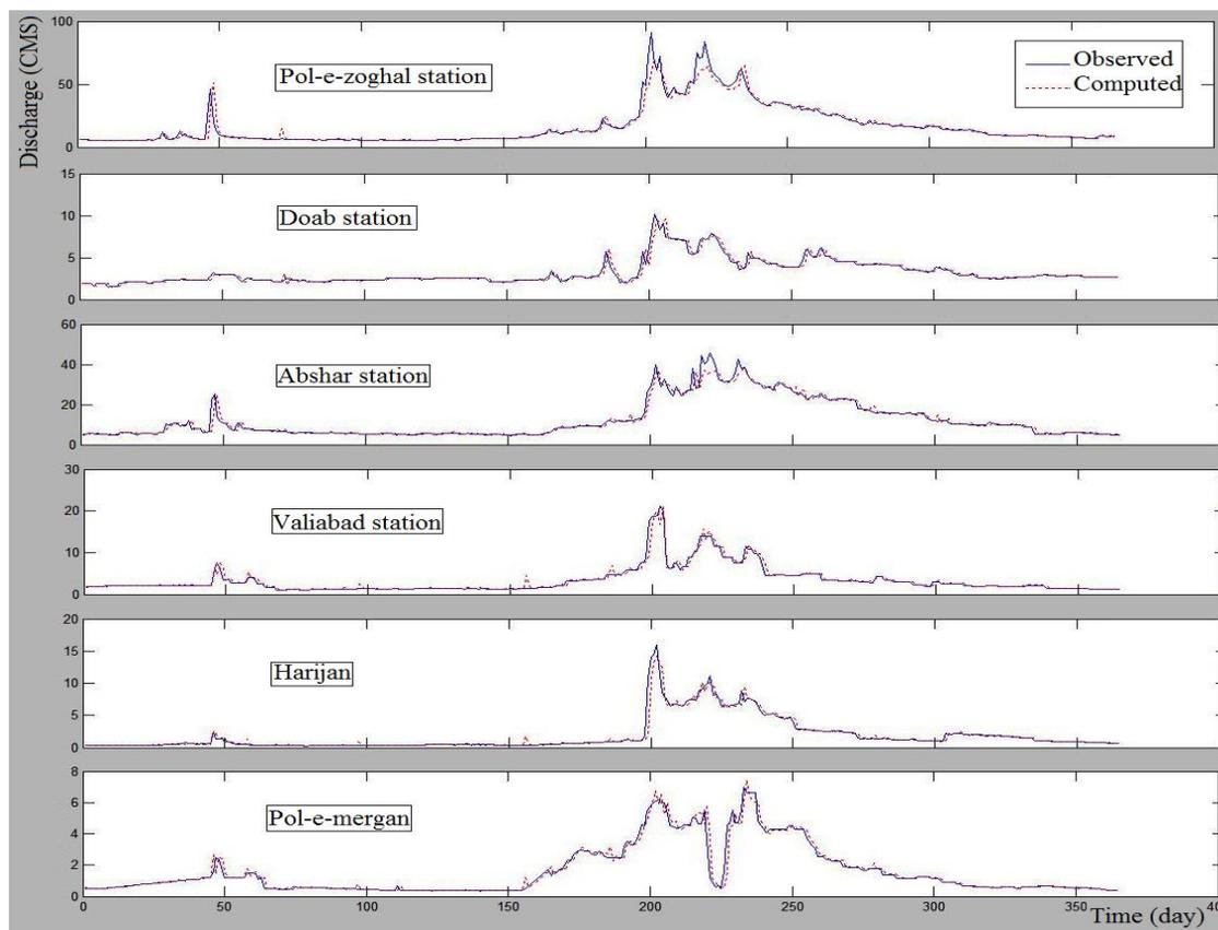
Fig. 4. Comparison of computed and observed of the last year (validation period) of the IGANFIS model.
