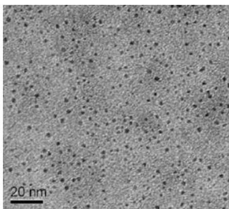
**Fig. 1.** TEM micrographs of Cu-NPs.
