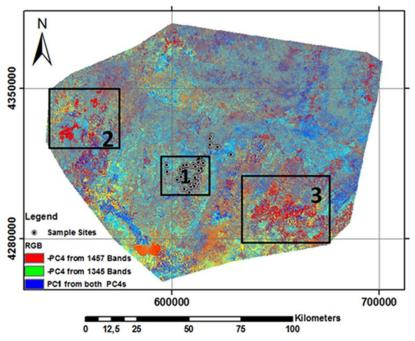
Fig. 7. Final false color composite image consisting of -PC4 from PCA of 1<sup>st</sup>, 4<sup>th</sup>, 5<sup>th</sup> and 7<sup>th</sup> bands (R), -PC4 from PCA of 1<sup>st</sup>, 3<sup>rd</sup>, 4<sup>th</sup> and 5<sup>th</sup> bands (G) and PC1 from PCA of both PC4 images (B).
