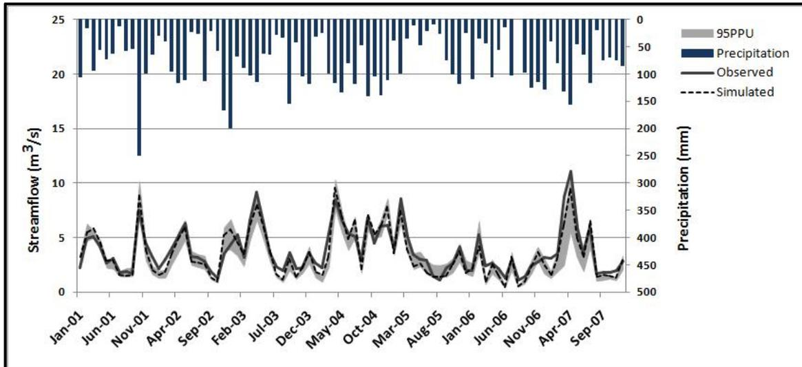
Fig. 3. 95% probability uncertainty plot and comparison observed and simulated streamflow after calibration (2001-2007).
