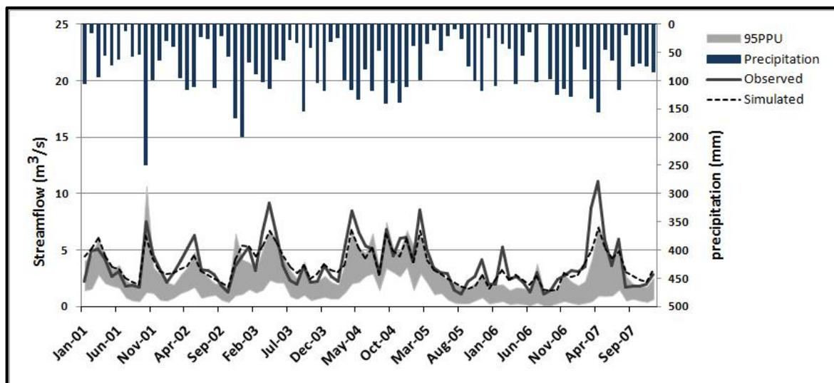
**Fig. 2.** 95% probability of uncertainty plot and comparing observed and simulated streamflow before calibration.
