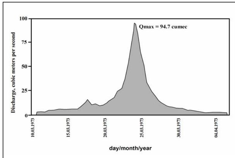
**Fig 4.** Discharge hydrograph of March 19 – 28, 1973 for Glavacioc River
